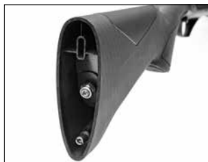
Remove the stock insert.
