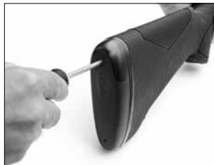
Insert a screwdriver into the holes in the recoil pad.
