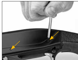
Push the trigger group pins through the receiver.
