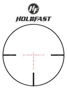
The Nikko Stirling HOLDFAST reticle has been developed to take longer distance shots quickly by using HOLDFAST lines that match the known point of impact of popular ammunition. A wide variety of ammunition can be accurately used when you adjust the image size in relation to the HOLDFAST reticle by simply adjusting the Magnification Power.
