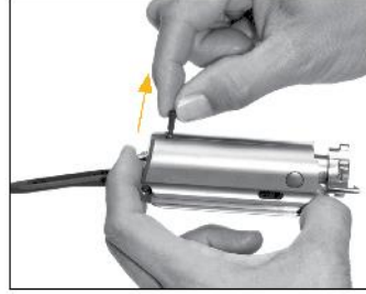
Remove the firing pin retaining pin.
