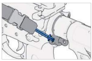
*Fig. 65: Thread in carrying sling with quick-release*
