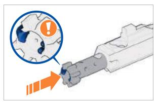
*Fig. 118: Insert bolt head into bolt head carrier*
