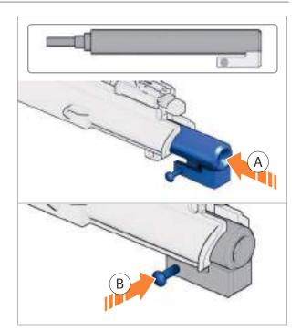
*Fig. 106: Insert cleaning rod guide*
