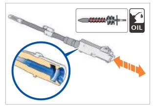
Fig. 110: Clean chamber and locking piece
