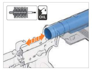
Fig. 104: Lubricate inside extension
