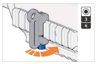
*Fig. 55:* Insert adapter for carrying sling on Picatinny rail
