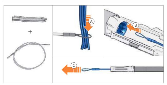
Fig. 112: Clean barrel with cleaning string
