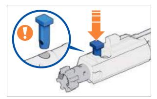
*Fig. 119: Insert control bolt*
