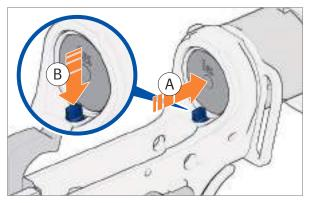
Fig. 95: Push in locking pin for buffer
