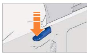
Fig. 21: Pressing right bolt catch/ release
