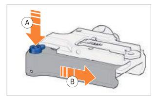
*Fig. 73:* Push locking device to the rear and hold
