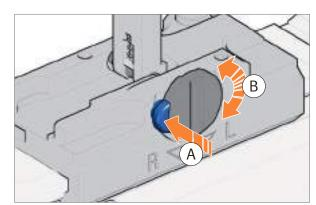
Fig. 81: Turn the windage adjustment screw
