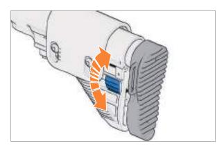
*Fig. 50: Turning the extension wheel*
