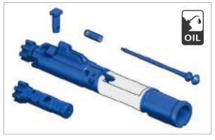
Fig. 115: Lubrication points of bolt group
