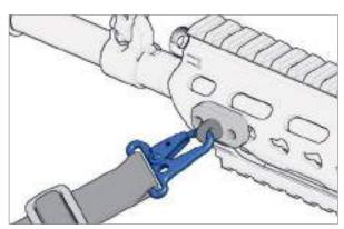
Fig. 59: Attach carrying sling with snaphook
