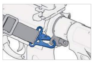
*Fig. 63: Attach carrying sling with snaphook*
