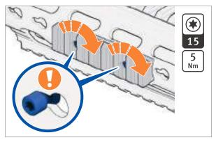
*Fig. 45: Tighten screws for Picatinny rail*
