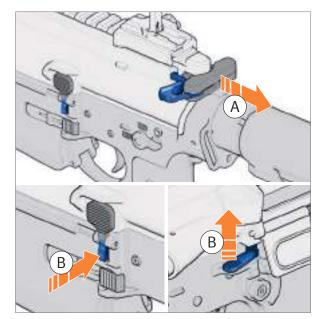
Fig. 18: Lock bolt group into place
