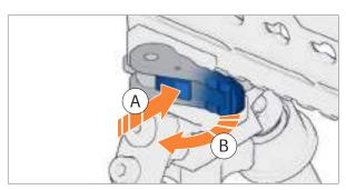
Fig. 36: Remove bipod
