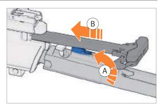
*Fig. 123:* Inserting bolt group into charging handle
