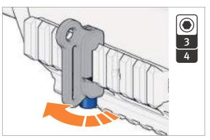
Fig. 56: Remove adapter for carrying sling
