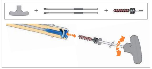
Fig. 105: Using the T-pistol grip
