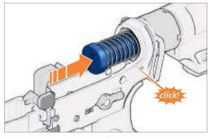
*Fig. 124: Insert buffer with recoil spring into buttstock*
