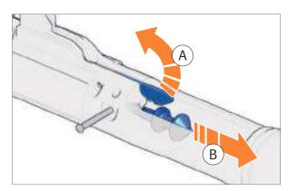
*Fig. 100: Remove firing pin and pressure spring for firing pin*
