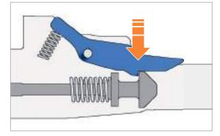
Fig. 9: Firing pin safety
