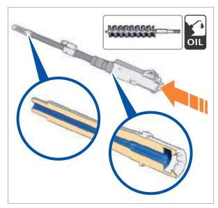
Fig. 111: Lubricate the inside of the barrel
