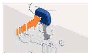
*Fig. 20: Pressing left bolt catch/release*
