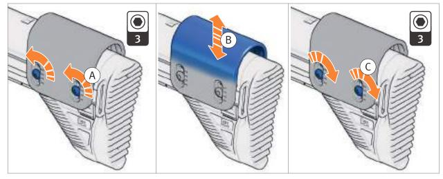
*Fig. 49:* Loosen screws with Allen key
