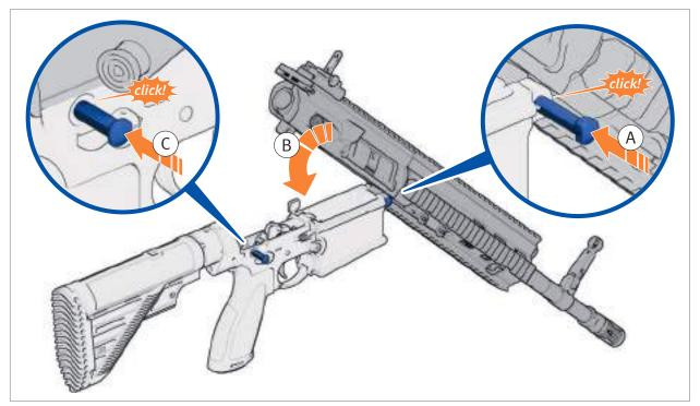
*Fig. 125: Insert lower receiver*
