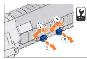
Fig. 91: Unscrew locking screw for handguard
