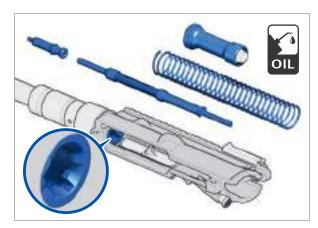
*Fig. 117: Lubrication points of functional elements*
