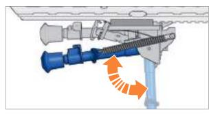
*Fig. 43: Fold out bipod / fold in bipod*
