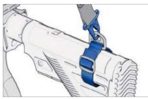
Fig. 66: Attach carrying sling to buttstock collar
