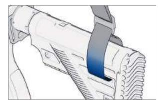
Fig. 67: Thread carrying sling directly
