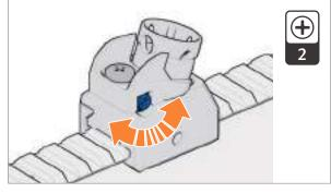
Fig. 84: Turn the windage adjustment screw
