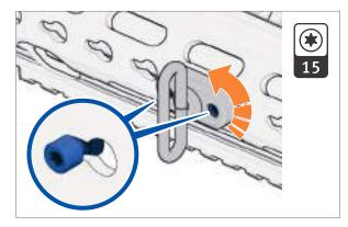
Fig. 52: Remove adapter for carrying sling
