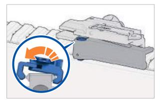
*Fig. 74: Insert quick-release sight*
