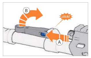
*Fig. 72: Unfold front sight*
