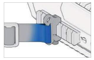
*Fig. 62: Thread carrying sling directly*
