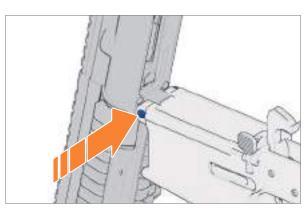
*Fig. 94: Push in front locking pin*
