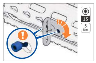
*Fig. 51:* Insert adapter for carrying sling into HKey interface
