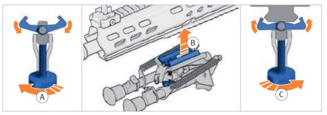
Fig. 42: Insert bipod
