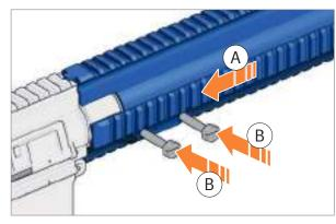
Fig. 126: Push handguard onto barrel
