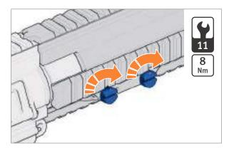
Fig. 127: Tightening locking screw for handguard
