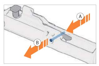
*Fig. 99:* Pull locking pin out of bolt head carrier
