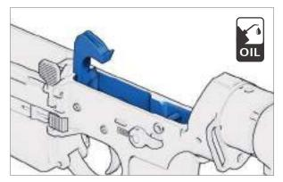
*Fig. 116: Lubrication points on lower receiver*
