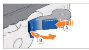
*Fig. 41: Remove bipod*
