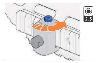
Fig. 54: Remove adapter for carrying sling
