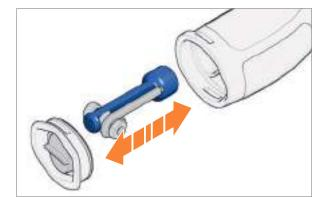
Fig. 25: Insert / remove multi-purpose tool
