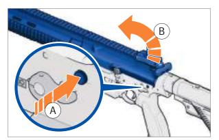
*Fig. 93: Push in rear locking pin*
