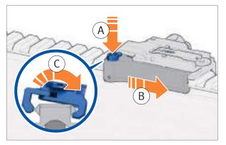
*Fig. 75: Remove quick-release sight*
