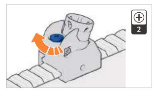
*Fig. 85: Tighten the locking screw*
