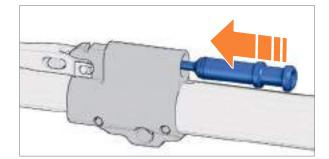
Fig. 121: Insert gas piston
