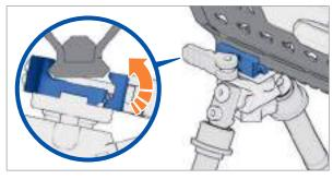
Fig. 32: Insert bipod
