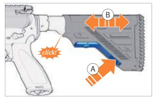
*Fig. 47: Adjust buttstock*
