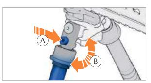
Fig. 34: Fold / unfold bipod
