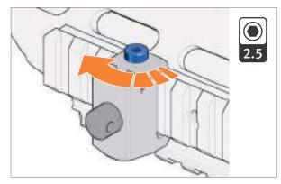
*Fig. 53:* Insert adapter for carrying sling on Picatinny rail
