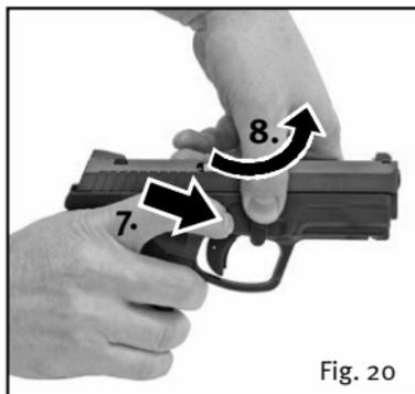
7 Press the integrated limited access lock in with the index finger of your firing hand and hold it pressed in.
