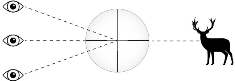
ing conditions or type of ammunition, use the height adjustment (6) and the lateral adjustment (7). No movement of the reticle is perceptible during reticle adjustment. The reticle is therefore always located in the center of the image. The reticle adjustment of the riflescope is performed as follows:
