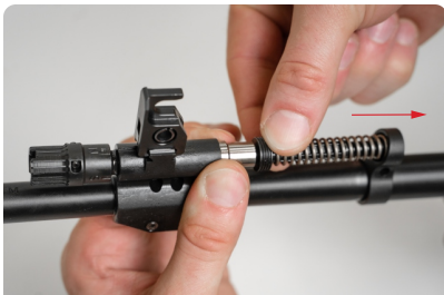
Figure 19 - Tirer la tige du piston
